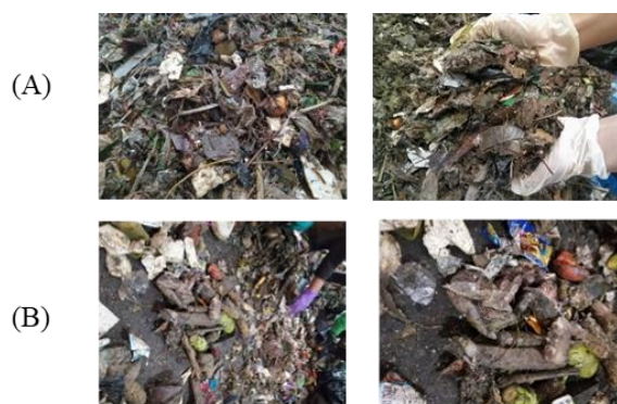
Figure 2. Rejected materials from the MSW separation plant: (A) rejected material 1 is a fine rejected fraction passing through a 50 mm dynamic disc screen, and (B) rejected material 2 refers to the dense rejected fraction passing through a 100 mm dynamic disc screen and subjected to a wind sifter.
