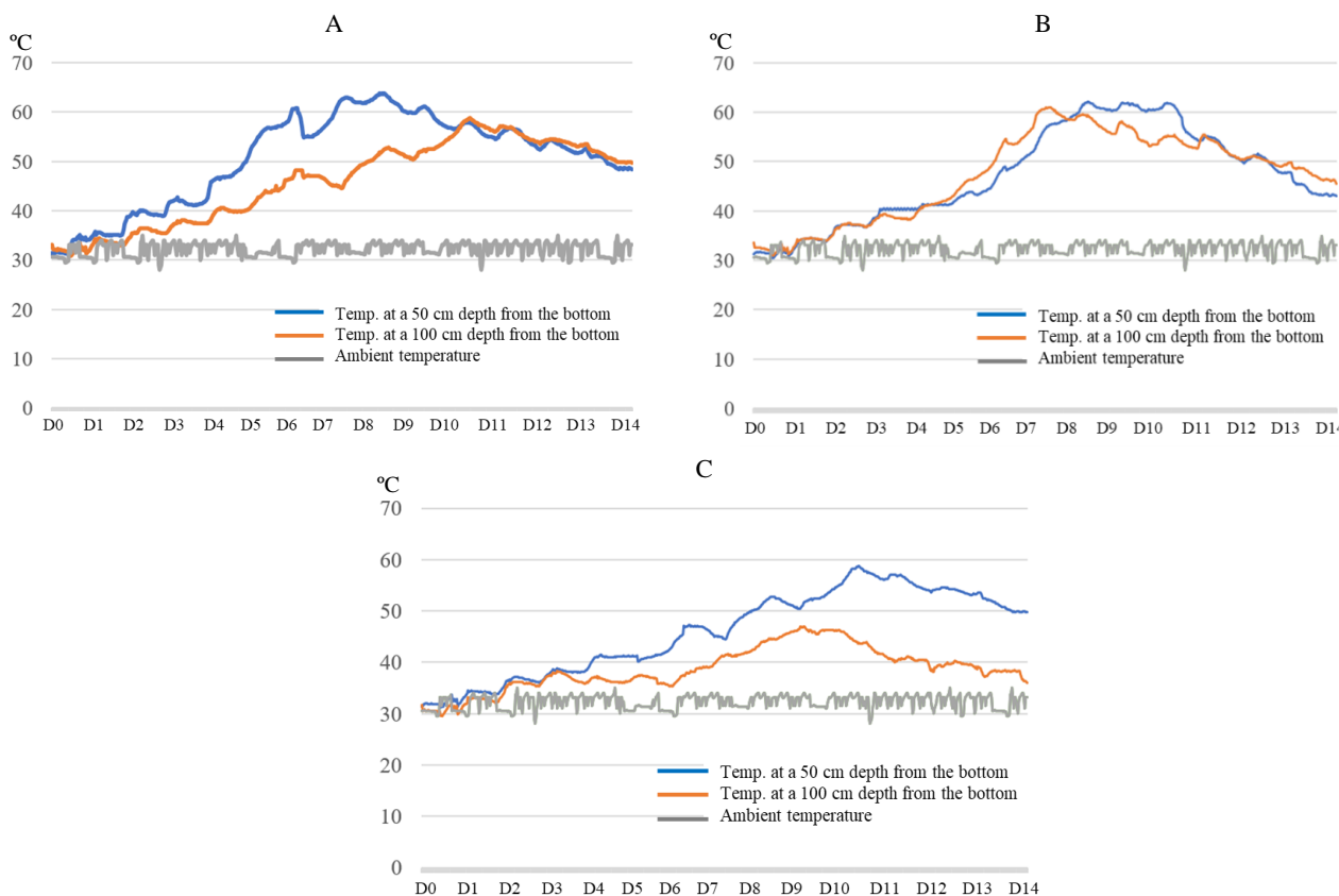
Figure 4. Daily average temperature (at a depth of 50 and 100 cm from the bottom) during the bio-drying process of the MSW rejected material 1 at different aeration rates: (A) T1 (B) T2 and (C) T3.
